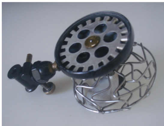
Trico vacuum fan with back cover removed
